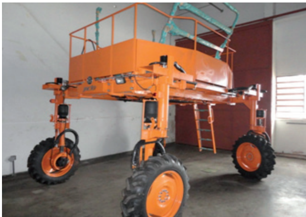
Fig. 2. AgriBOT prototype. Photo of the robot when it was delivered by Jacto company in December 2010
