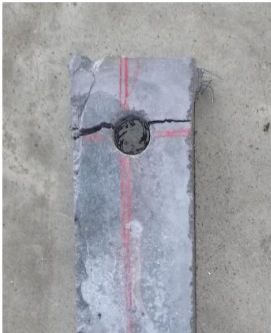
Figure 3. Net tension failure.
